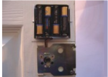
Step 10. Picture shows battery pack installed into the battery casing
