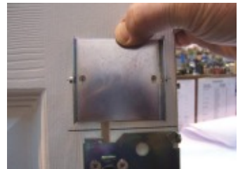
Step 9. Shows the battery pack inner casing plate being aligned to its position
