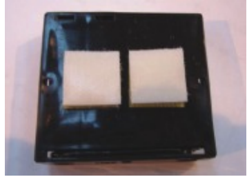
Step 10. Picture shows adhesive pads in inner battery casing
