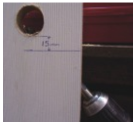
Step 14. Drill the angled path for the battery leads
