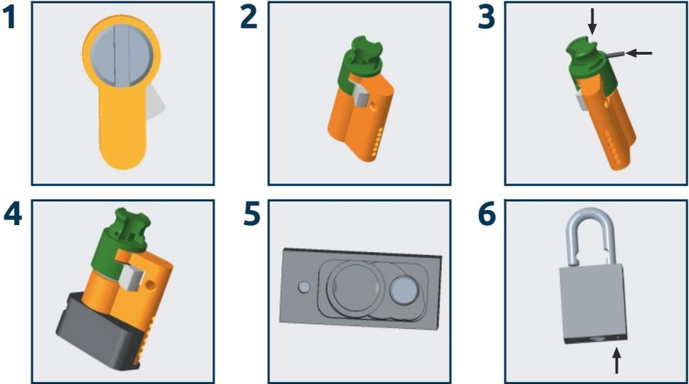
1. The half euro cylinder required for this lock must be 45mm long (35mm to the centre of the cam) and, when looking at the front, the cam must be protruding to the right. (see Pic 1)
