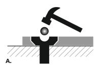
Hammer the anti-drill steel balls into the top of the socket heads.
